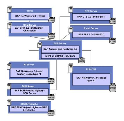
We do not recommend installing all components on one host. Instead you can distribute the components among several hosts, as shown in the diagram above. The diagram provides just one example; there are several ways to distribute the components. The distribution depends on many factors, such as sizing, security, available hardware, and so on. In practice, any distribution of components among hosts is possible.
